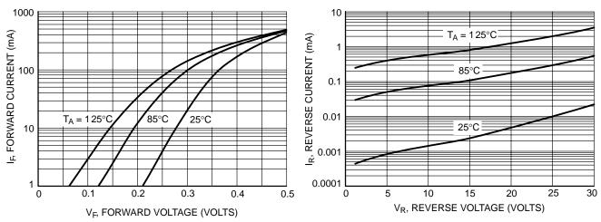
Figure 2. Forward Current as a Function of Forward Voltage; Typical Values
